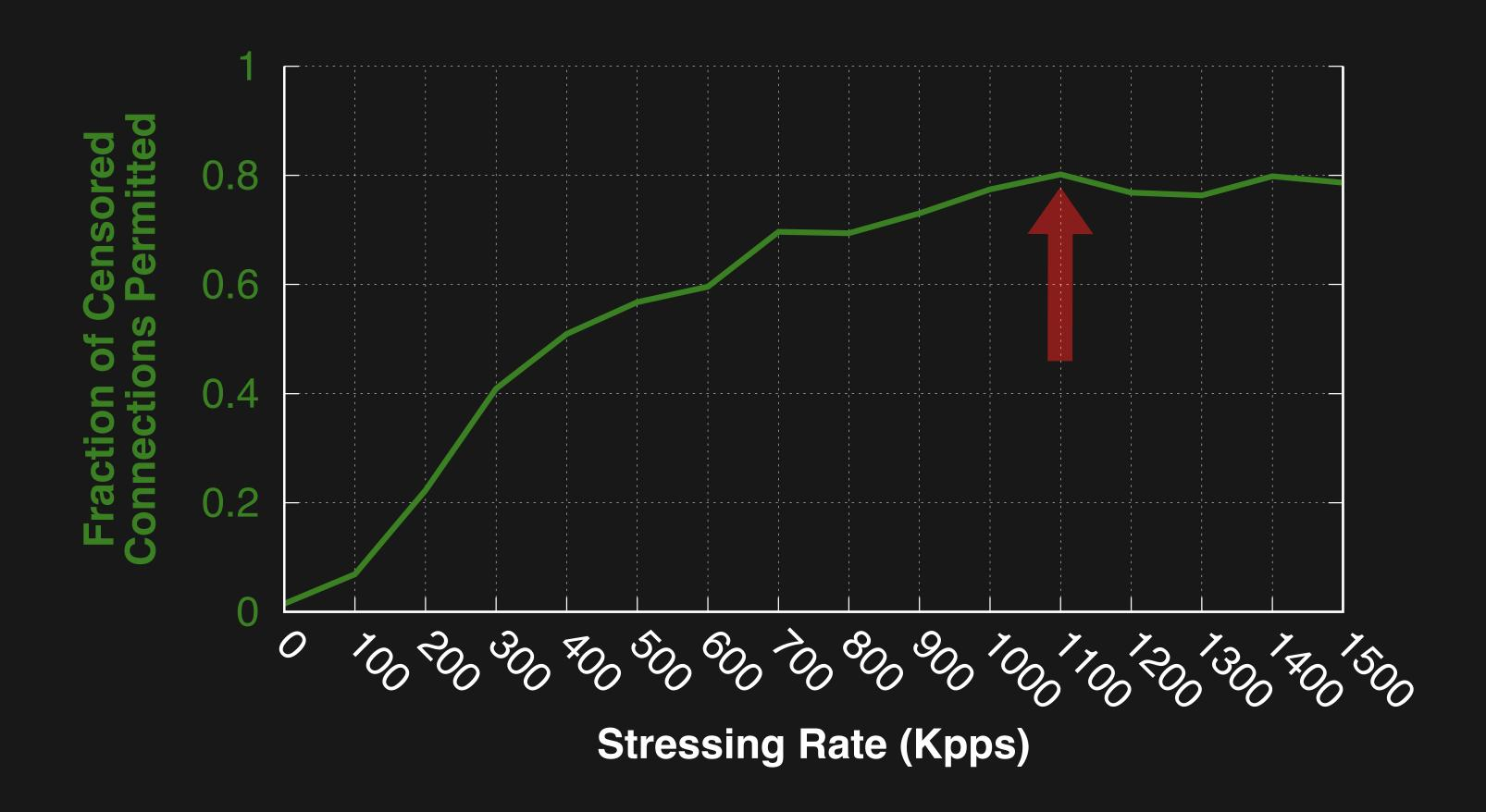
The GFW failed to censor 80% of QUIC connections under moderate-load conditions.
