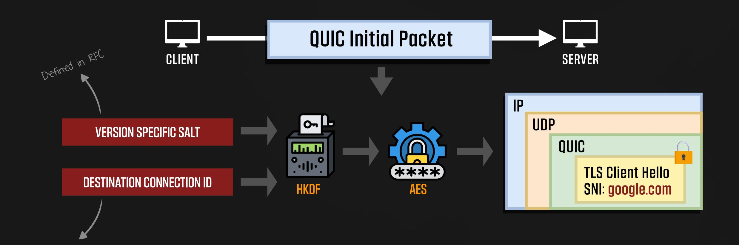
Encrypted with a key that is derivable by a passive observer
